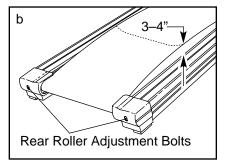
belt centered. Plug in the power cord, insert the key and run the treadmill for a few minutes. Repeat until the walking belt is properly tightened.
